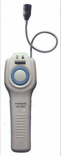
Combustible Gas Leak Detector
