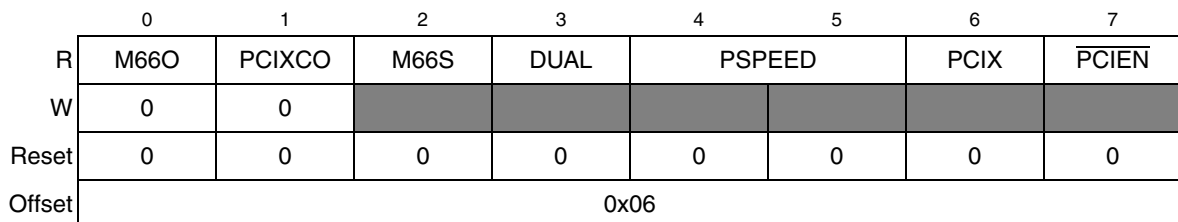
Figure 3-7. PCI Control/Status Register (CM_PCI)
