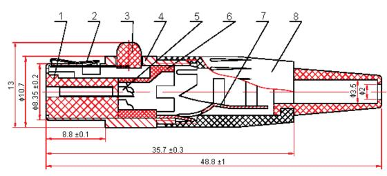
The female pin plating gold, thickness 0.05μm (SOLDER).
