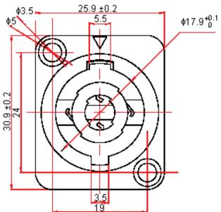
The pin plating gold, thickness 0.05µm (SOLDER).
