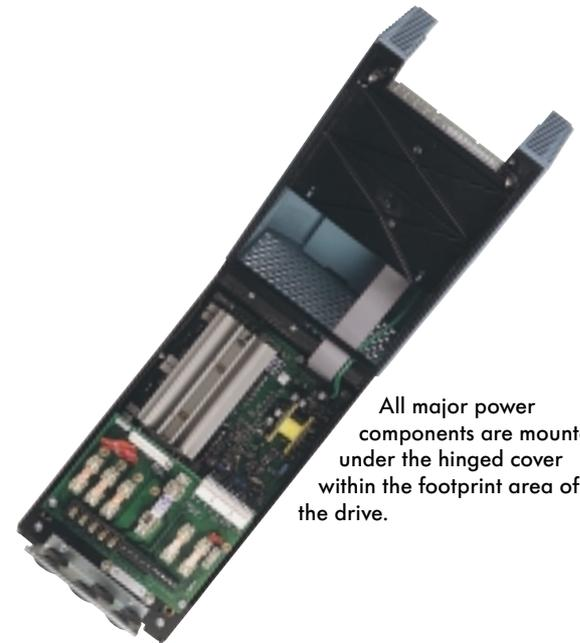
All major power components are mounted under the hinged cover within the footprint area of the drive.
