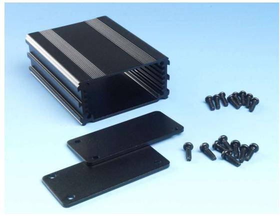
Part Number: B1-080 EX SERIES 1 ENCLOSURE Extruded aluminum case kit with 2 end panels and assembly screws – 1.18 H x 2.5 W x 3.15 L" / deep Size: 1.18H x 2.5W x 3.15L" Battery Type: N/A Product Name: BEX SERIES 1 ENCLOSURE Size: 1.18Hx2.5Wx3.15L" Weight in Pounds: 0.4 Material: Aluminum 6063 T6 (HE9)
