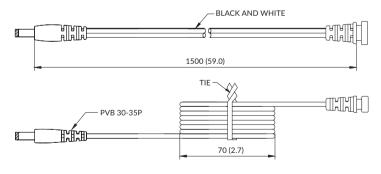
Wire type: VW-1  $80^{\circ}\text{C}$  300 V L=1500 mm 2464 24 AWG 2C Black and White. Black - Negative, White - Positive
