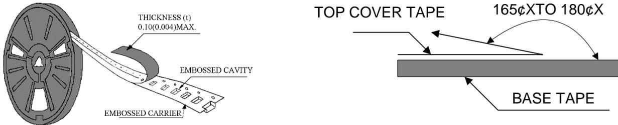
The force for peeling of cover tape is 10 grams in the arrow direction.
