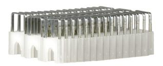
Jonard Tools No. 19 1/4-inch by 1/4-inch clear insulated cable staples are genuine Jonard fasteners, designed for use with the <u>STG-100</u> <u>TriggerTack™</u> wire and cable tacker. Each box has 300 pieces, and is ideal for installing security wire (18/4), telephone wire 24/8), thermostat wire (18/2, 18/5, 18/8), and Ethernet Cat-5 voice and data cable.
