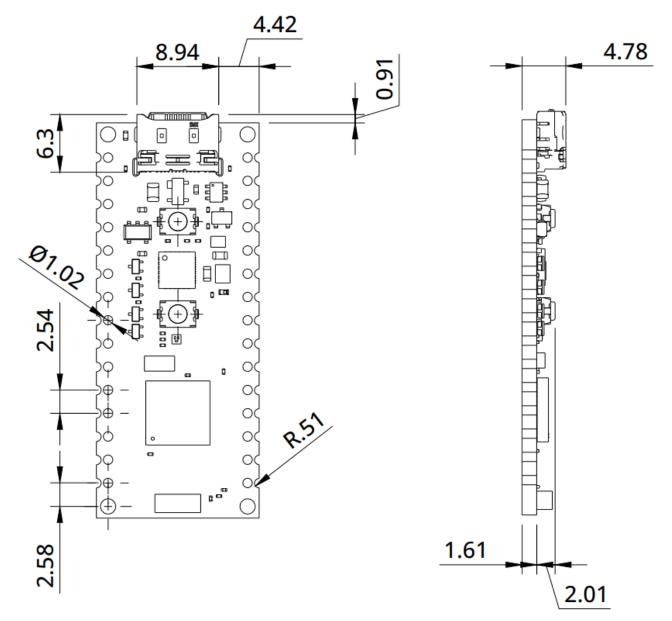
The Nano Matter was designed to be usable as a surface-mount module and presents a dual inline package (DIP) format with the Nano-styled header connectors on a 2.54 mm pitch grid with 1 mm holes.
