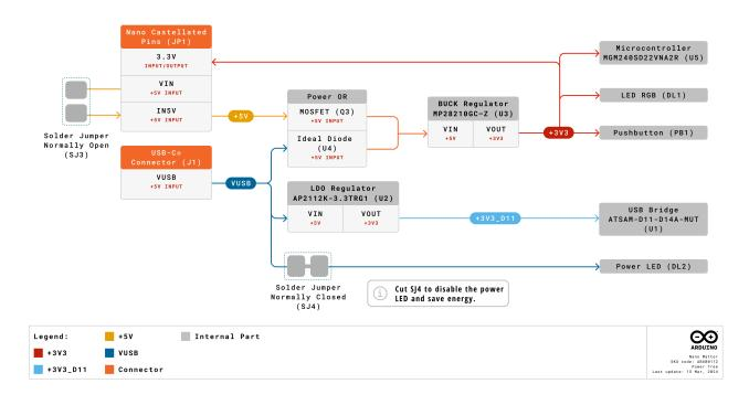
**Low-Power Tip:** For power efficiency, safely cut the LED jumper and connect an external +3.3 VDC power supply to the board's 3V3 pin. This configuration does not power the board's USB bridge.
