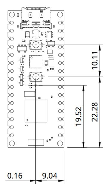
The Nano Matter is designed to be usable as a surface-mount module and presents a dual inline package (DIP) format with the Nano-styled header connectors on a 2.54 mm pitch grid with 1 mm holes.
