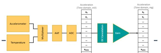
When the system requests a data measurement, the sensor acquires 4096 data points at the required bandwidth. The information below shows the relationship between sampling frequency, bandwidth, and acquisition duration (warm-up and processing times are not included):
