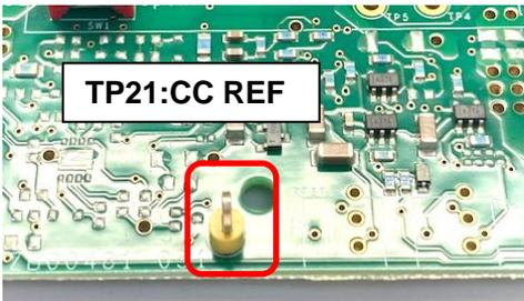
Inject signal from Output Source into TP21. This is reference signal for constant current.
