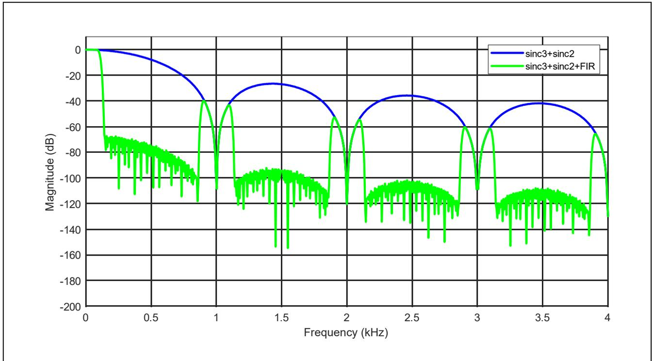
**Figure 15** Combined output of the Back End
