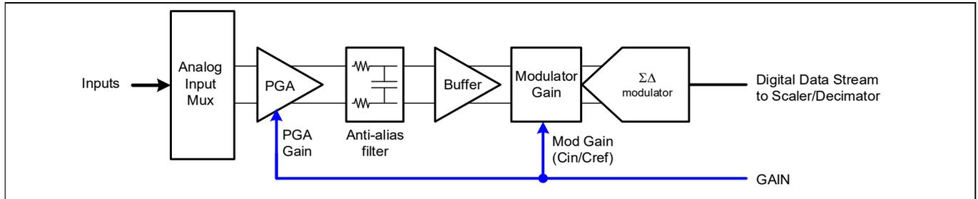
**Figure 8** Analog DSM channel
