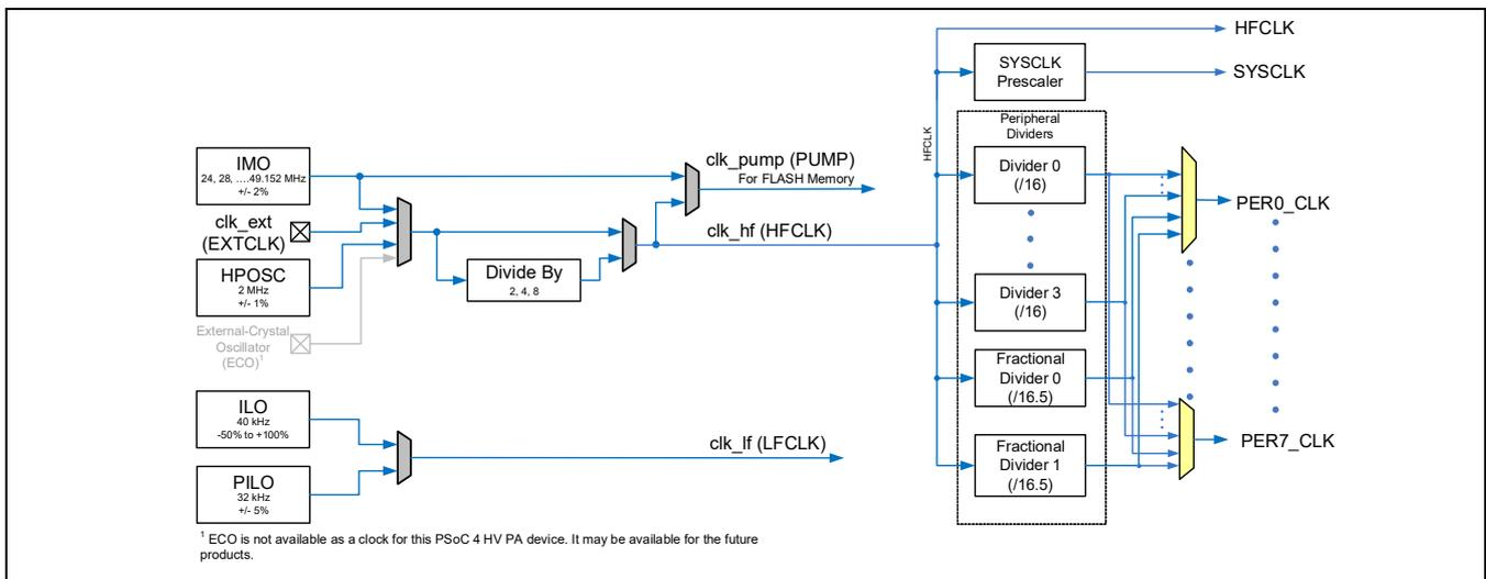
**Figure 2 PSoC™ 4 HV PA clocking architecture**
