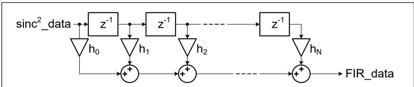
**Figure 14** **General structure of the FIR filter**
