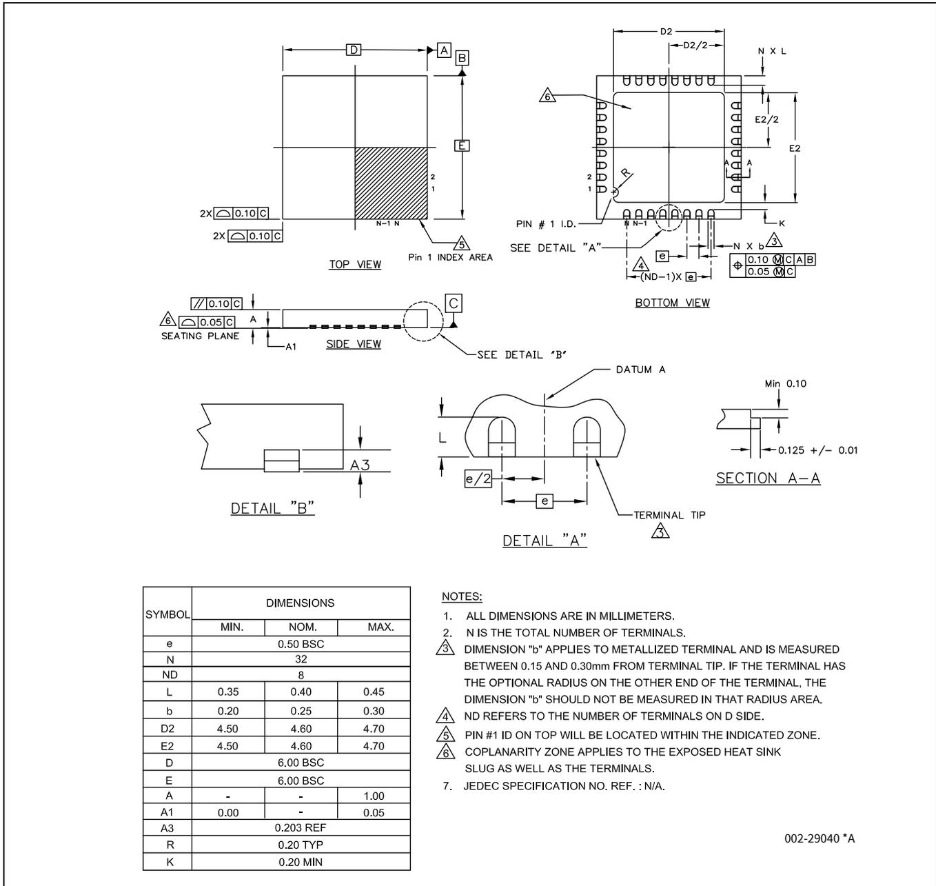
Figure 24 32-Pin QFN with wettable flank (6.0 x 6.0 x 1 mm)
