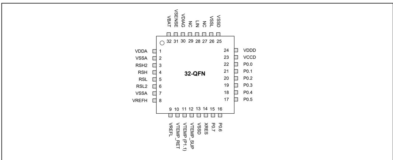
**Figure 23 Pin assignment**
