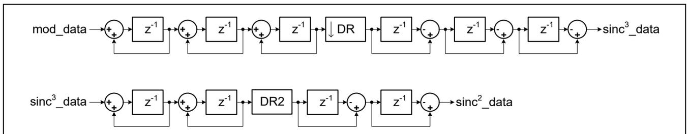
**Figure 12 Block diagram of sinc3 and sinc2 decimators**
