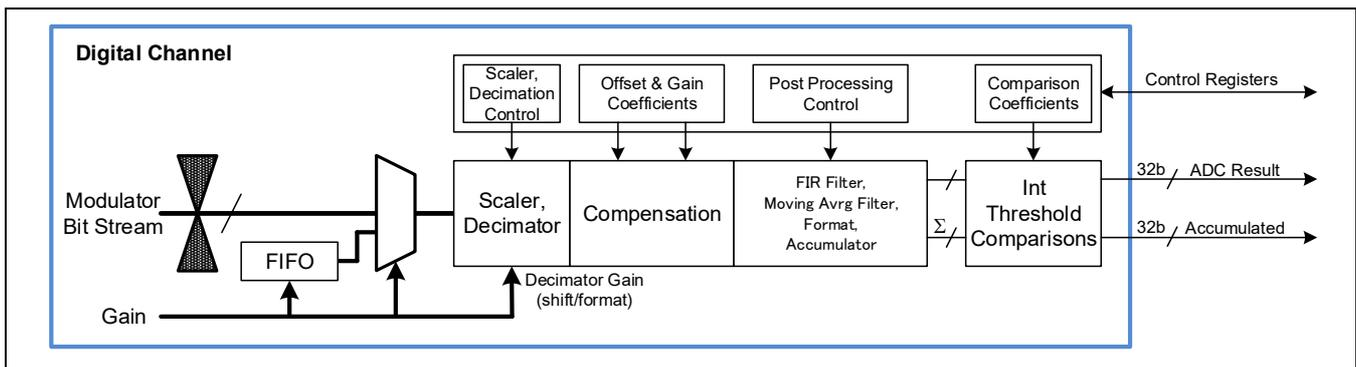
**Figure 10** Digital channel data path
