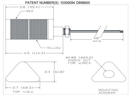
LED OPERATION: CONNECT STACK COLOR WIRE TO POWER AND BROWN WIRE TO POWER.
