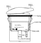
**Dimensions : Millimetres** Tolerance: ±0.5mm
