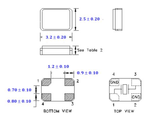
Note: Due to material availability, the chamfer could be located on pin #1, 3, or 4. Be advised that the chamfer location has no impact on the electrical performance of the device.
