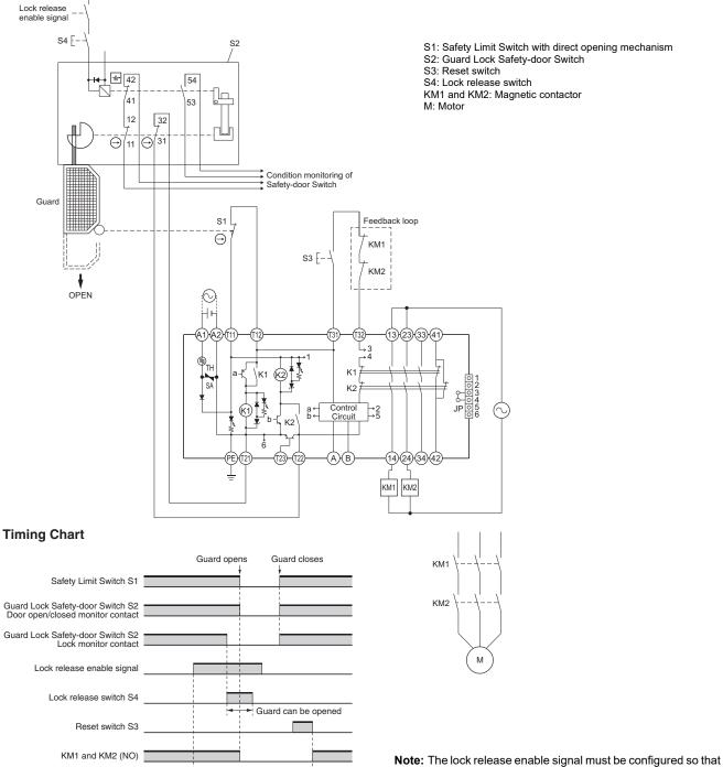
**lote:** The lock release enable signal must be configured so that it should turn ON after dangerous movement is stopped and safety is ensured for the door to open.
