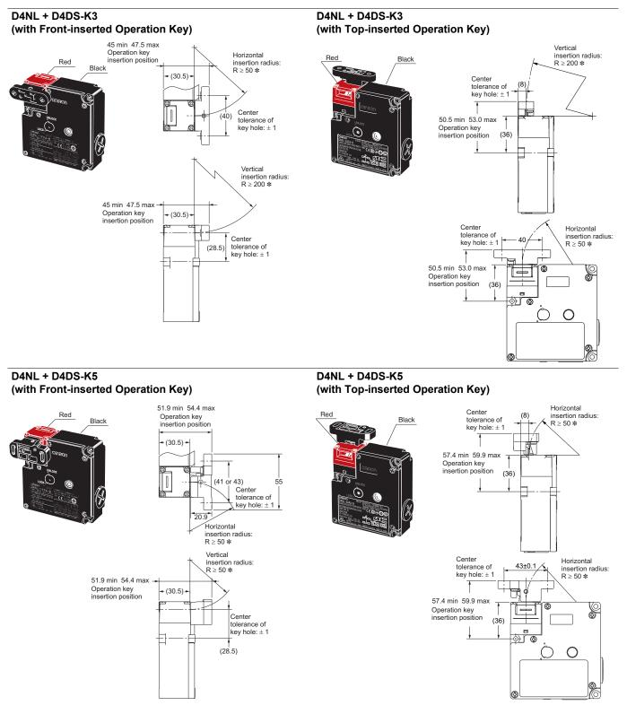
\* Insertion radii apply when the rotational center of the Operation Key is in line with a line extending from the front or top Head surface.
