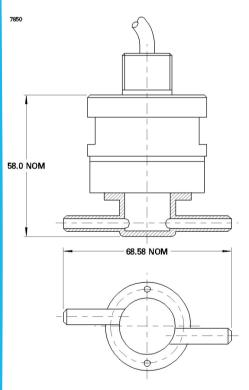
The Quick Calibration Hood is constructed from polypropylene, and provides a convenient means of supplying test gases to the VQ600 in the field, for calibration and checking purposes. The assembly push-fits into the central gas access recess of the head, and is designed to accommodate 6 mm ID or ¼" flexible tubing.
