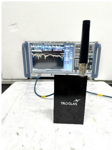
VNA Test Set-up – 9x15cm Ground Plane
