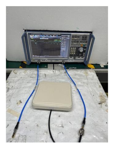
VNA Test Set-up
