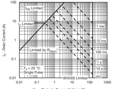
$V_{DS}$  - Drain-to-Source Voltage (V) \*  $V_{GS}$  > minimum  $V_{GS}$  at which  $R_{DS(on)}$  is specified
