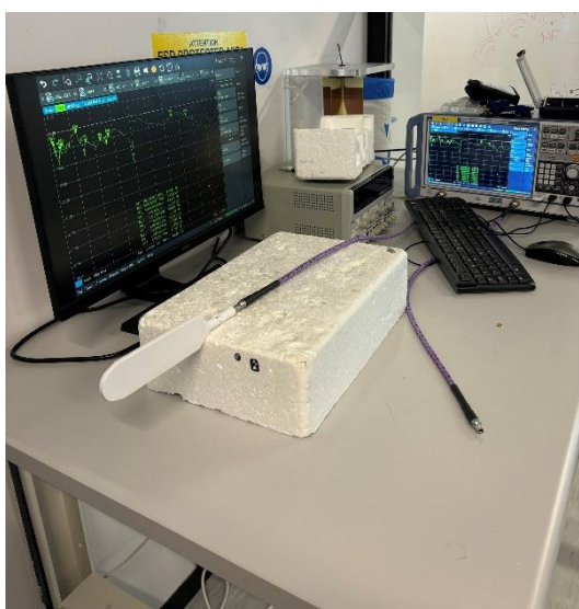
VNA Set up Straight in Free Space
