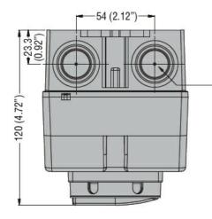
PG13.5 / M20 PG16 / M25 knockouts on top and bottom **GAZ032**
