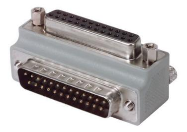
Connecting cables in tight spaces can be a problem in many applications. These low profile right angle D-Sub adapters solve this problem by allowing cab 90 degree angle. Three versions are available for each connector size allowing for cables to exit in opposite directions. Adapters are male to female, fully overmolded with gray PVC. Mating hardware is reversible allowing for use in virtually any application.
