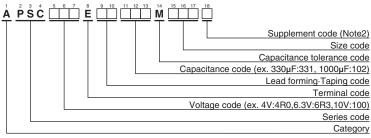
(Note2) PSC series, 2.5V820µF(ESR 5mΩ max.) has supplement code "J". Can case, terminal and terminal plating are the same as all others in PSC series.
