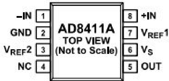
Figure 4. 8-Lead MSOP and 8-Lead SOIC Pin Configuration
