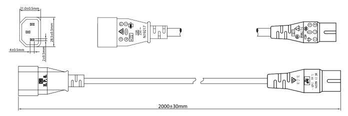
CABLE MARKING: H03VVH2-F 2X0.75mm² < VDE > N19626 60227 IEC 52 300/300V HIGH PROJECT CABLE COLOUR: BLACK
