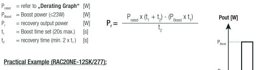
Take the RAC20NE-12SK/277at 230VAC input Voltage and full load at  $\rm T_{\rm AMB}{=}$  80°C ,with natural convection.
