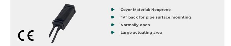
Internal lever switches are designed for manual actuation applications, where a larger actuator area with more travel is required. Encased in neoprene rubber, these basic switches feature a "V" shape back for pipe mounting.
