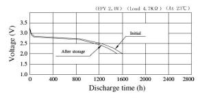
Storage at 60°C for 30 days equivalent to storage at room temperature for 18 months
