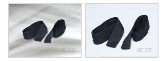
Tubing Product Type: Heat Shrink Tubing Primary Product Color: Black Shrink Ratio: 2:1 Recovered Inside Diameter (Max): 30 mm [ 1.181 in ] Primary Product Material: Polyethylene/Polyester
