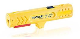
$\sim$  Cable stripper for longitudinal cut of sheathing of PUR-coated fibre optic cables  $\sim$  Opening the sheathing of PUR-coated fibre optic cables with longitudinal cut  $\sim$  Working range: Ø 6,2 mm  $\sim$  with durable and Features & Benefits
