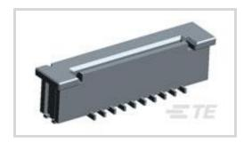
Centerline (Pitch): .5 mm [ .02 in ] Mating Retention Type: Zero Insertion Force (ZIF) PCB Mount Orientation: Vertical Termination Method to PCB: Surface Mount FPC Actuator Type: Stuffer
