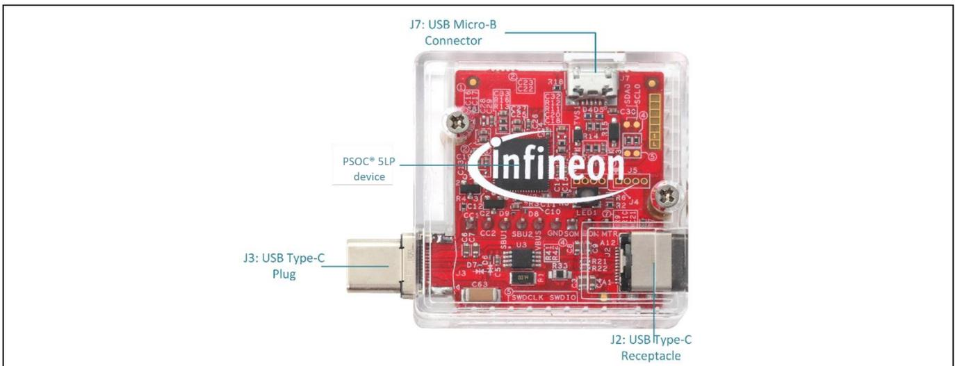
**Figure 2** CY4500-EPR EZ-PD™ Protocol Analyzer board (front view)
