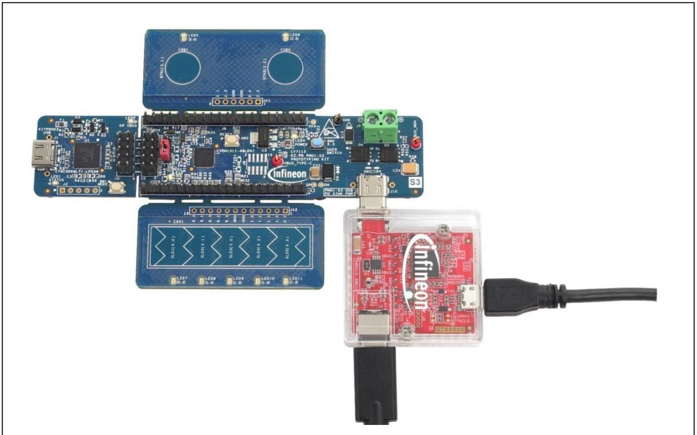
Figure 13 Complete setup of CY4500-EPR EZ-PD™ Protocol Analyzer
