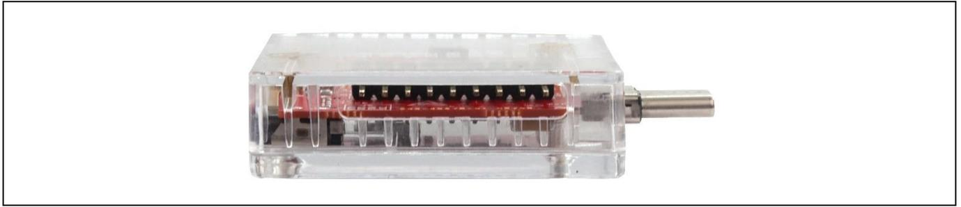
Figure 4 CY4500-EPR EZ-PD™ Protocol Analyzer board (side view)
