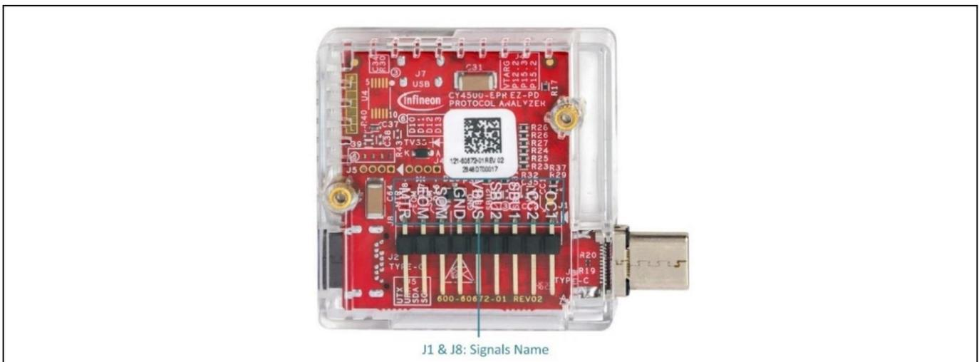
**Figure 3** CY4500-EPR EZ-PD™ Protocol Analyzer board (rear view)
