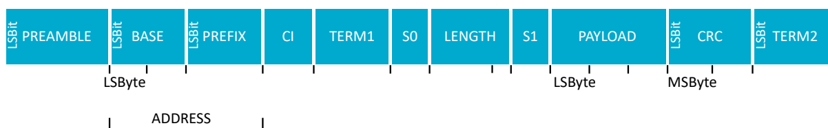
Figure 109: On-air packet layout for Long Range (125 kbps and 500 kbps) Bluetooth Low Energy modes
