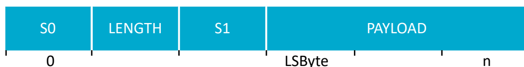
Figure 110: Representation of a RADIO packet in RAM
