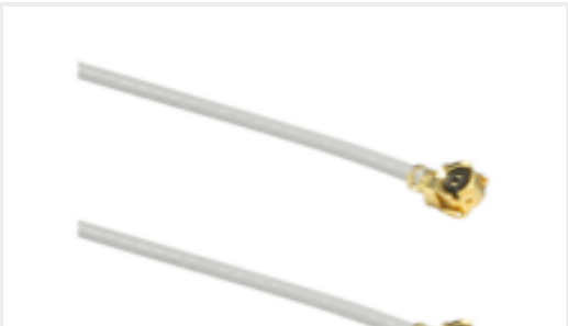
TE Part #CSI-UFFR-100-UFFR U.FL/MHF1 to U.FL/MHF1 100mm 1.13 OD
