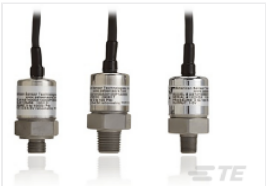
TE Part #11105403-00 10000 PSI, 7/16-20UNFM, 20 mV/V, 2ft Cbl
