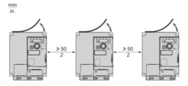
Free space ≥ 50 mm (2 in.) on each side. Vent cover should be removed for operation at surrounding air temperature above 50 °C (122 °F). The degree of protection becomes IP20.
