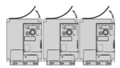
Drives mounted side-by-side, vent cover should be removed. The degree of protection becomes IP20.
