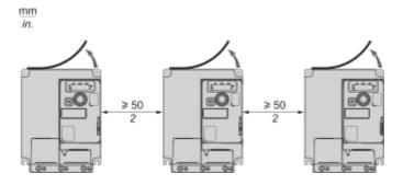
Free space ≥ 50 mm (2 in.) on each side. Vent cover should be removed for operation at surrounding air temperature above 50 °C (122 °F). The degree of protection becomes IP20.
