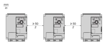
Free space ≥ 50 mm (2 in.) on each side, with vent cover fitted.
