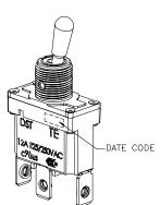
Single Pole Double Throw, Yellow Cap on Actuator, Screw Terminal
