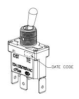
Single Pole Double Throw, Yellow Cap on Actuator, Quick Connect Terminal
