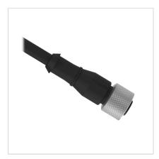
Cordset: Single Ended M12 8-pin Straight Female 16 m 8x24 Shielded Black PVC Jacket Nickel-Plated Brass Coupling Nut Part Number: 81538
