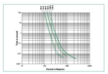
1. Rerating depicted in this curve is in addition to the standard derating of 25% for continuous operation.
