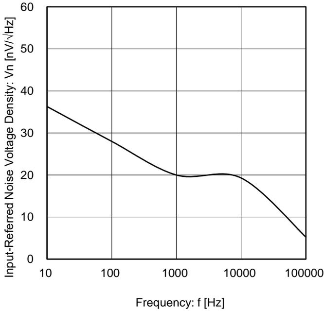
Figure 21. Input-Referred Noise Voltage Density vs Frequency (V<sub>DD</sub> = 5 V)
