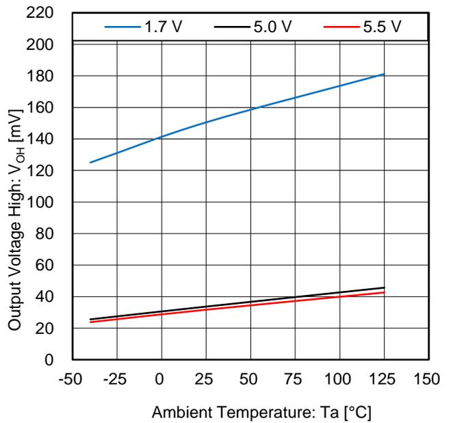
Figure 4. Output Voltage High vs Ambient Temperature
