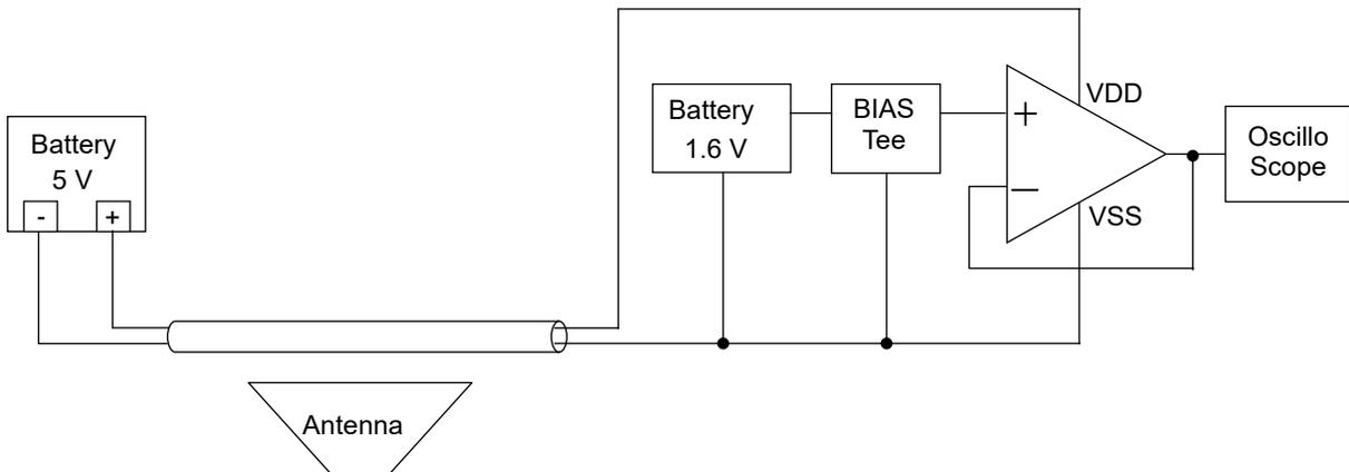
Figure 26. Measurement Circuit of EMI Evaluation
