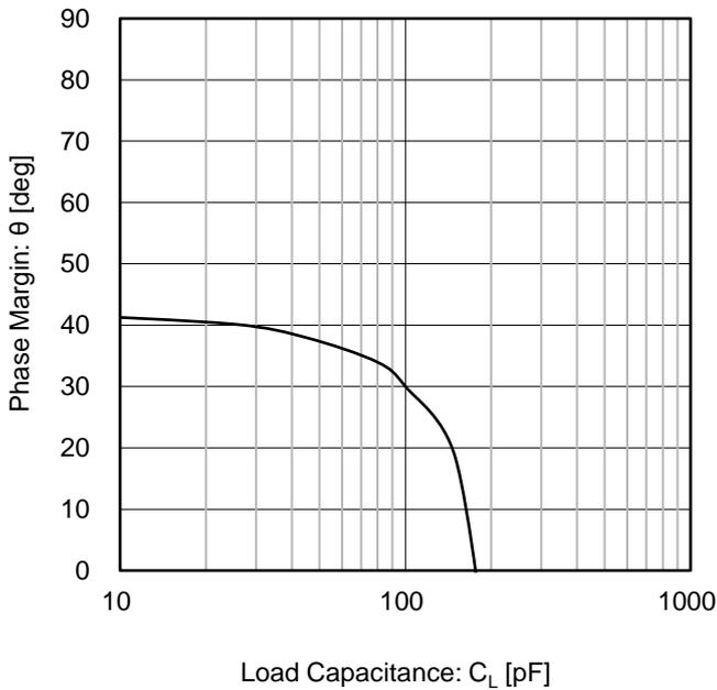
Figure 23. Phase Margin vs Load Capacitance (V<sub>DD</sub> = 5 V, G = 40 dB)
