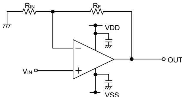
Figure 30. Non-inverting Amplifier Circuit
