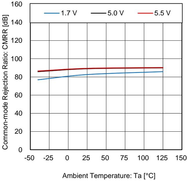
Figure 17. Common-mode Rejection Ratio vs Ambient Temperature
