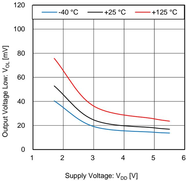
Figure 5. Output Voltage Low vs Supply Voltage ( $I_{OUT} = 1\text{ mA}$ )
