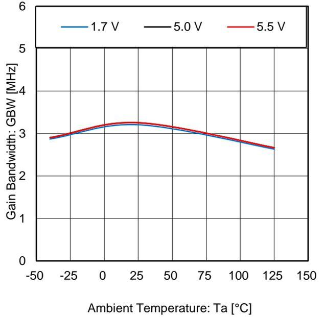
Figure 22. Gain Bandwidth vs Ambient Temperature
