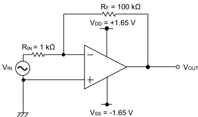
$$V_{OUT} = -\frac{R_F}{R_{IN}} V_{IN}$$
