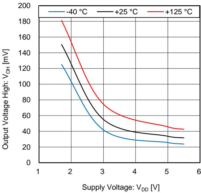
Figure 3. Output Voltage High vs Supply Voltage
