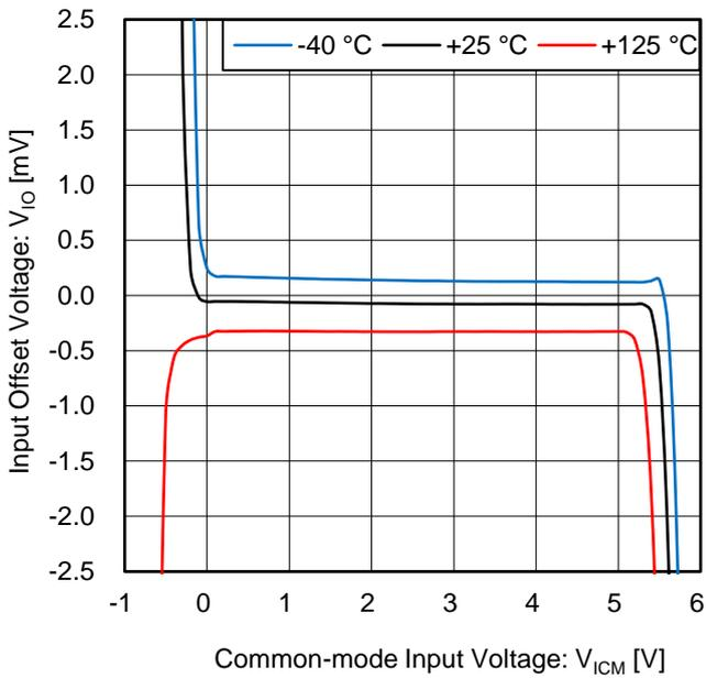
Figure 13. Input Offset Voltage vs Common-mode Input Voltage
