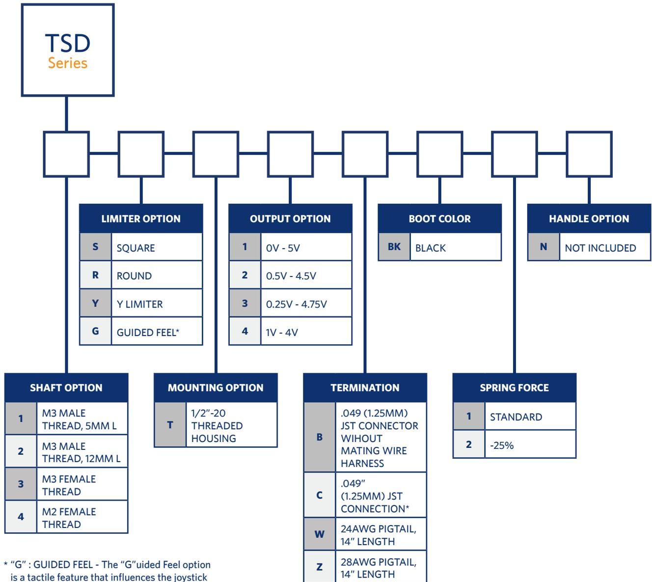
\* "G" : GUIDED FEEL - The "G"uided Feel option is a tactile feature that influences the joystick movement into the cardinal (N,S,E,W) directions. The Guided Feel option allows for 360° movement throughout the diagonal positions, but actuation into the N,S,E,W positions is more refined.
