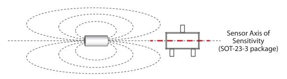
**Note:** The most straightforward way of aligning a magnet with a TMR sensor is by lining up the magnet's magnetization axis with the sensor's Axis of Sensitivity (as shown above). However, there are many other alignments and orientations that will also achieve proper operation. For any questions, or to learn more, please contact Coto Technology.
