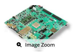
and a Mali<sup>™</sup>-400 MP2 graphics processing unit based on 16nm FinFET+ programmable logic fabric by AMD. The ZCU102 supports all major peripherals and interfaces, enabling development for a wide range of applications.
