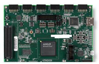
The SP701 Evaluation Kit, equipped with the best-in-class performance-per-watt AMD Spartan™ 7 FPGA, is built for designs requiring sensor fusion such as industrial networking, embedded vision, and automotive applications. The SP701 features high I/O availability and I/O expansion capability via Pmods and FMC connectors, making it the largest IP development canvas for Spartan 7
