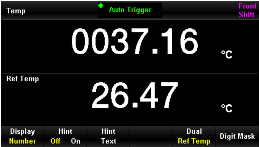
Figure 0-13 Dual Display of Temperature Measurement Menu 1
