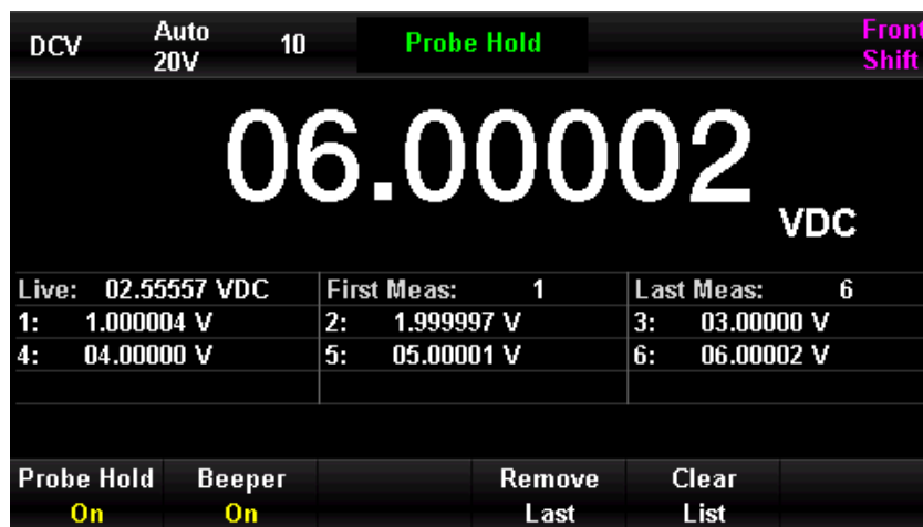
Figure 0-10 DCV Hold Measurement Menu
