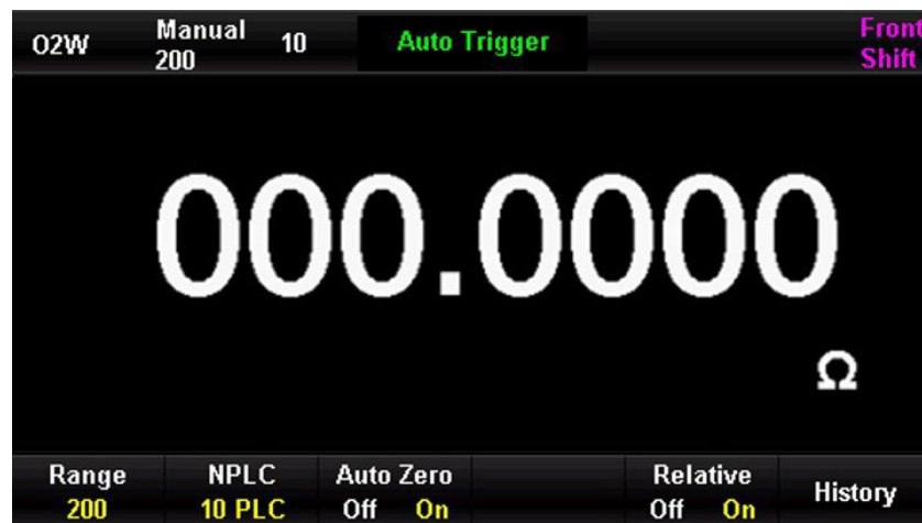
Figure 0-4 Resistance Reading after Relative Operation
