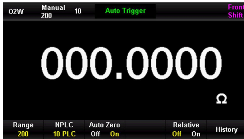
Figure 0-3 Reading of Test Wire Short-circuit
