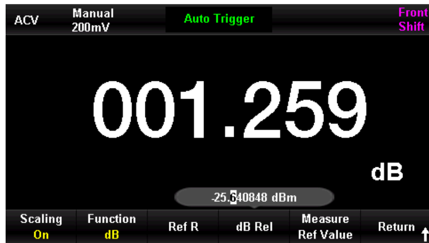
Figure 0-6 dB Measurement Menu
