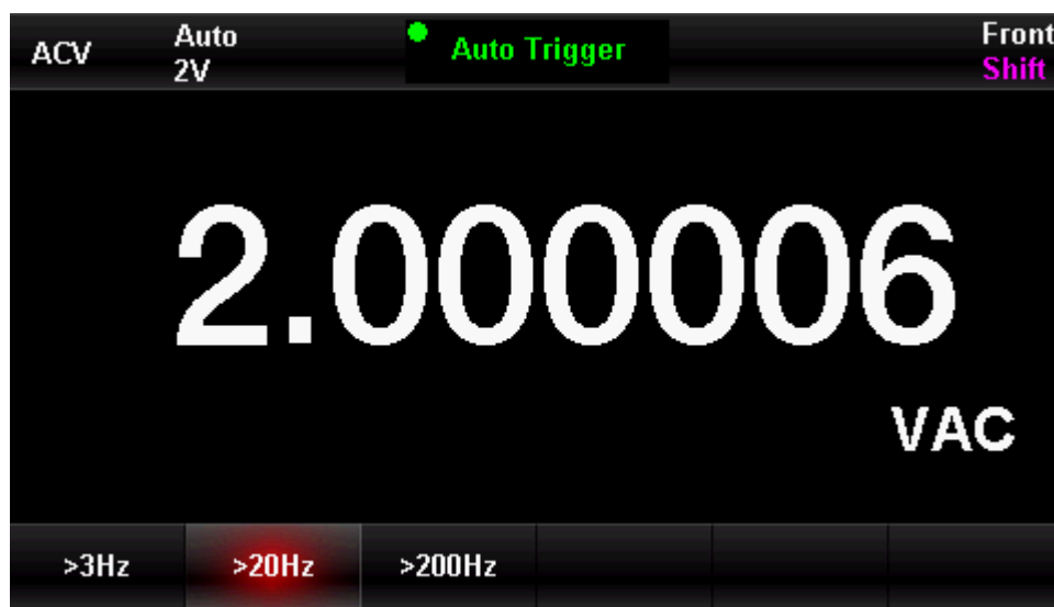
Figure 0-6 Low-frequency Filter Setting
