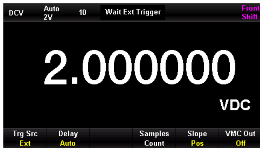
Figure 0–53 External Trigger Menu
