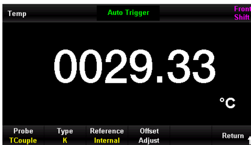
Figure 0–12 K-type Thermocouple Temperature Measurement Menu
