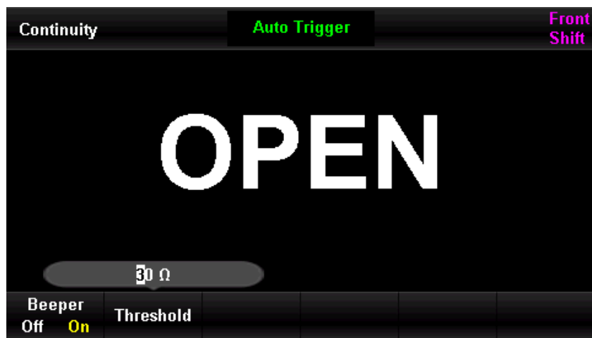
Figure 0–34 Continuity Measurement Menu
