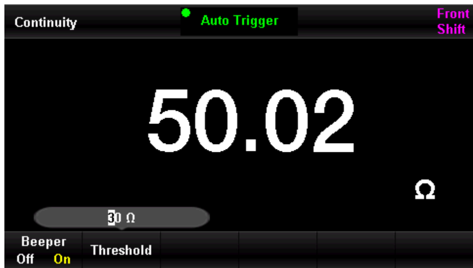
Figure 0-7 Short-circuit Resistance Setting
