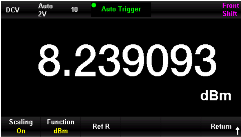
Figure 0-58 dBm Operation Menu
