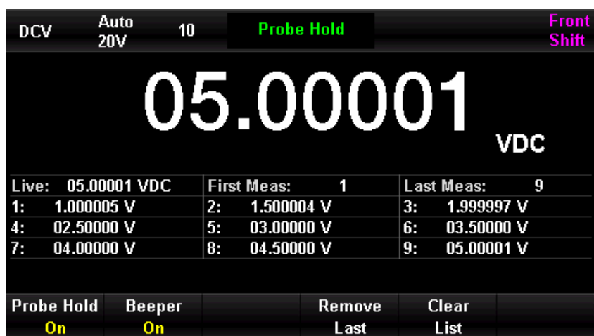
Figure 0-1 DCV Reading Statistics Menu 1
