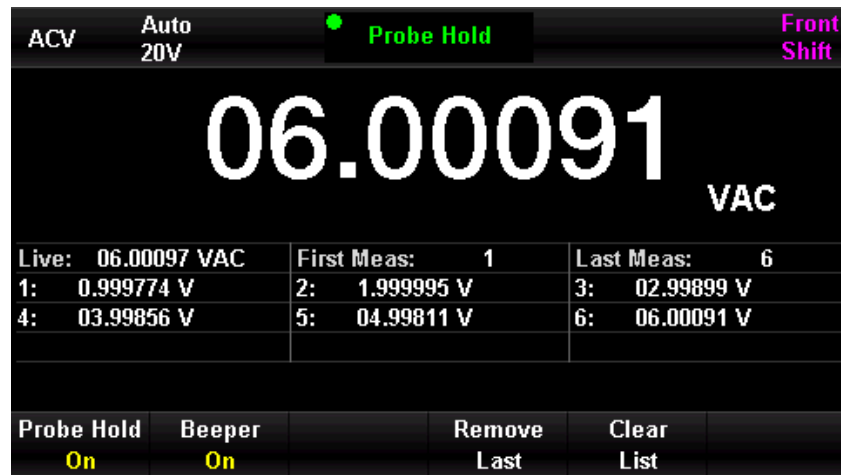
Figure 0-11 ACV Hold Measurement Menu
