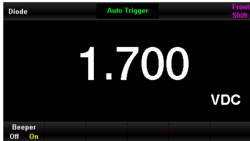
Figure 0–8 Diode Break-over Voltage Measurement
