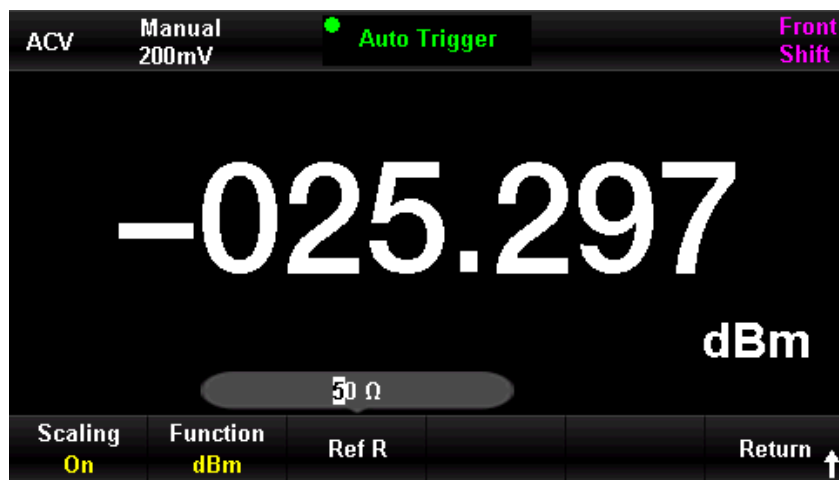
Figure 0-5 dBm Measurement Menu
