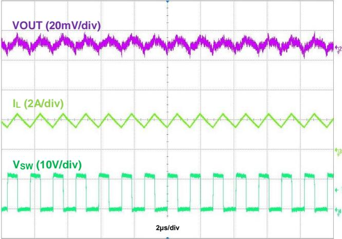
Figure 20. Output Voltage Ripple,  $V_{OUT} = 5\text{V}$ ,  $I_{OUT} = 2\text{A}$
