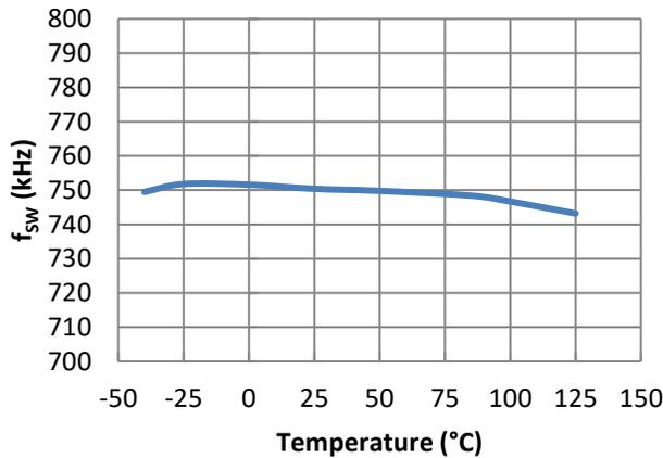
Figure 30.  $f_{sw}$  vs. Temperature,  $I_{OUT} = 0\text{A}$
