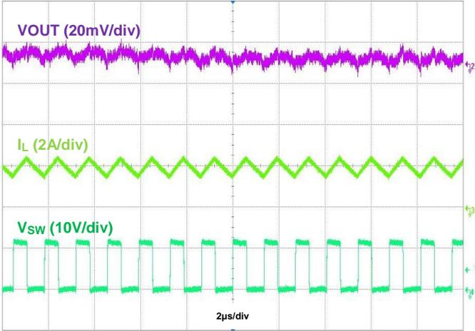
Figure 33. Output Voltage Ripple,  $V_{OUT} = 5\text{V}$ ,  $I_{OUT} = 2\text{A}$
