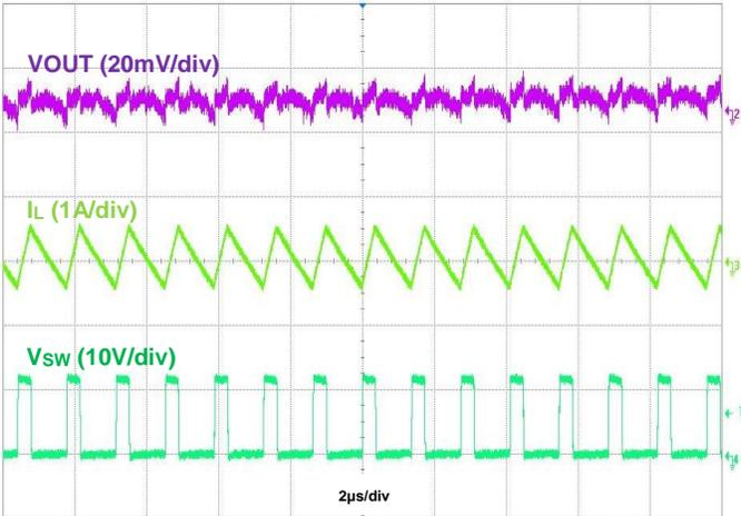
Figure 34. Output Voltage Ripple,  $V_{OUT} = 3.3\text{V}$ ,  $I_{OUT} = 50\text{mA}$
