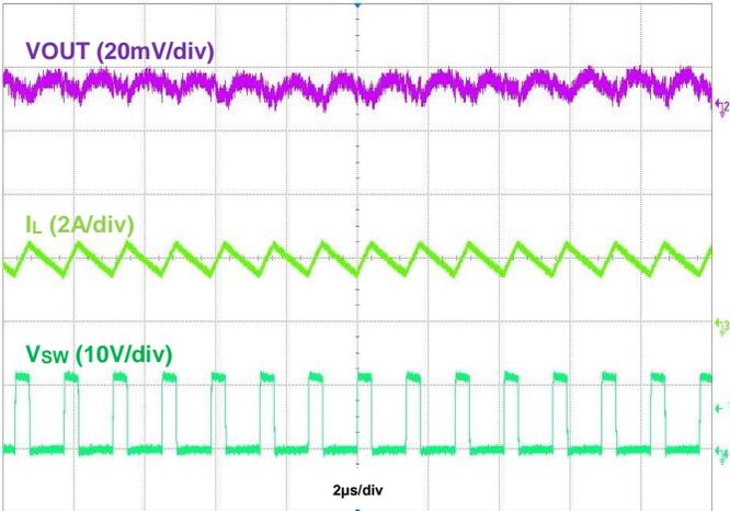
Figure 22. Output Voltage Ripple,  $V_{OUT} = 3.3\text{V}$ ,  $I_{OUT} = 2\text{A}$
