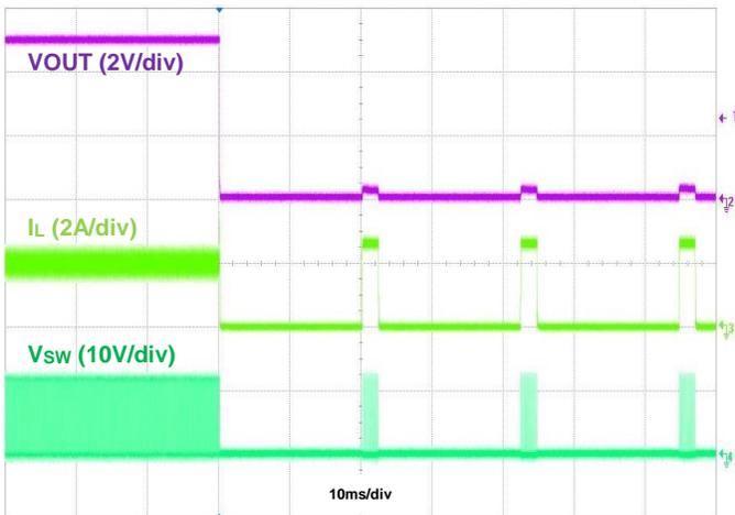
Figure 12. Output Short Protection, IOU = 2A
