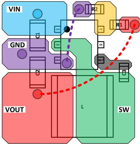
Figure 42. Recommended PCB Layout, SOT563 (Standard)
