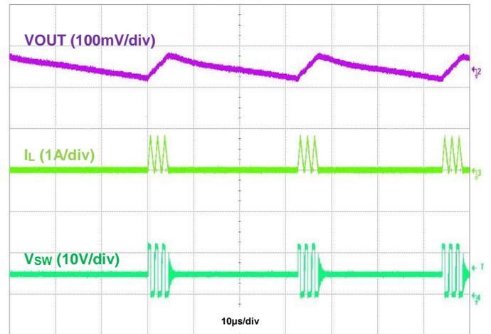
Figure 19. Output Voltage Ripple,  $V_{OUT} = 5\text{V}$ ,  $I_{OUT} = 50\text{mA}$
