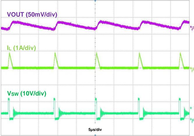
Figure 21. Output Voltage Ripple,  $V_{OUT} = 3.3\text{V}$ ,  $I_{OUT} = 50\text{mA}$
