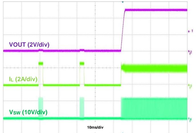
Figure 13. Output Short Recovery, IOU = 2A
