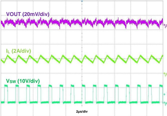
Figure 35. Output Voltage Ripple,  $V_{OUT} = 3.3\text{V}$ ,  $I_{OUT} = 2\text{A}$
