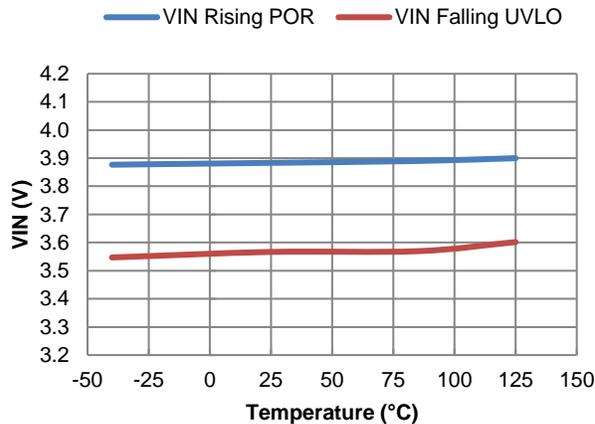
Figure 9. VIN Power-On Reset and UVLO vs. Temperature
