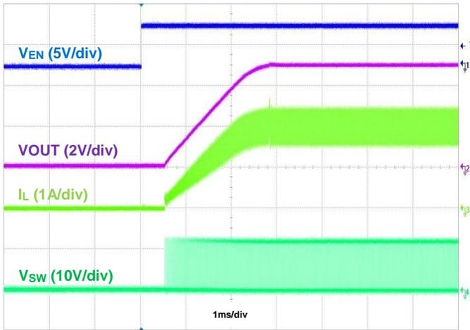
Figure 10. Startup Using EN, IOU = 2A
