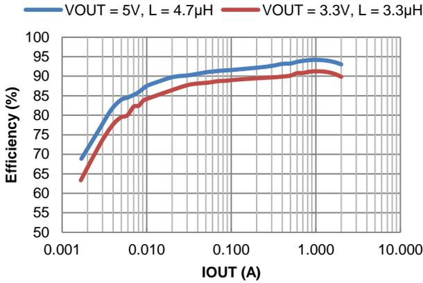
Figure 14. Efficiency vs. Output Current,  $V_{IN} = 12\text{V}$
