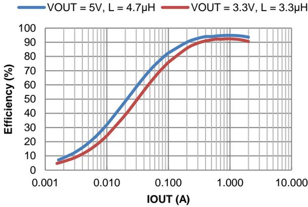
Figure 26. Efficiency vs. Output Current,  $V_{IN} = 12\text{V}$
