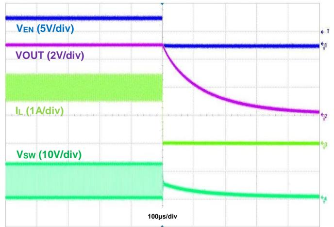
Figure 11. Shutdown Using EN, IOU = 2A
