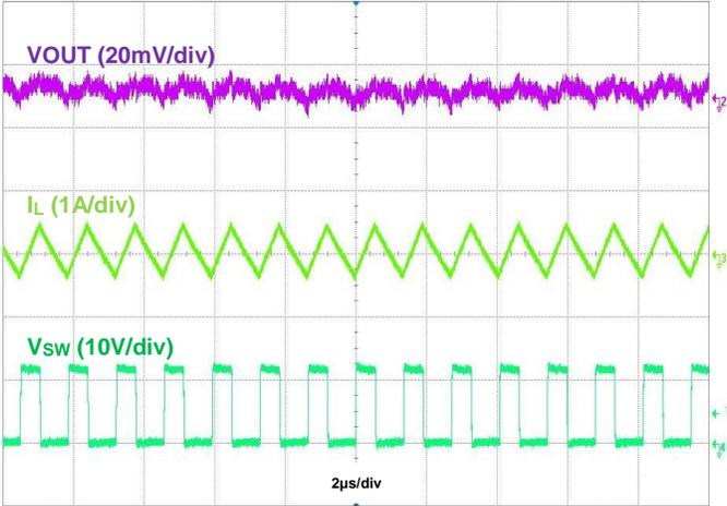
Figure 32. Output Voltage Ripple,  $V_{OUT} = 5\text{V}$ ,  $I_{OUT} = 50\text{mA}$
