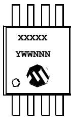
14-Lead SOIC (150 mil) (MCP6574)
